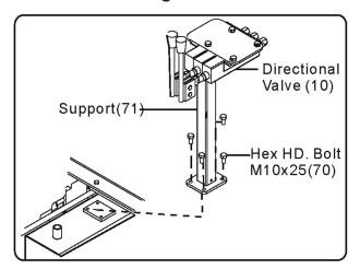
The control valve stand is attached onto the oil reservoir with 4 Hex Bolts (70) - See Figure C.
